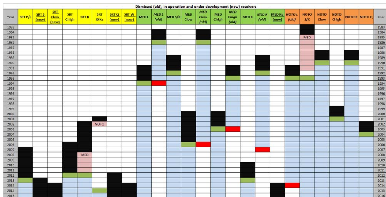
Figure 6.12 – Development duration for the receivers in operation, those under development (indicated with ‘new’) and the dismissed ones (‘old’). Black cells indicate the development period, the green cells the year of installation in its current radio telescope, the red cells the removal year, the light blue cells the operational period in its current radio telescope, and the orange cells the operational period in a different radio telescope.
