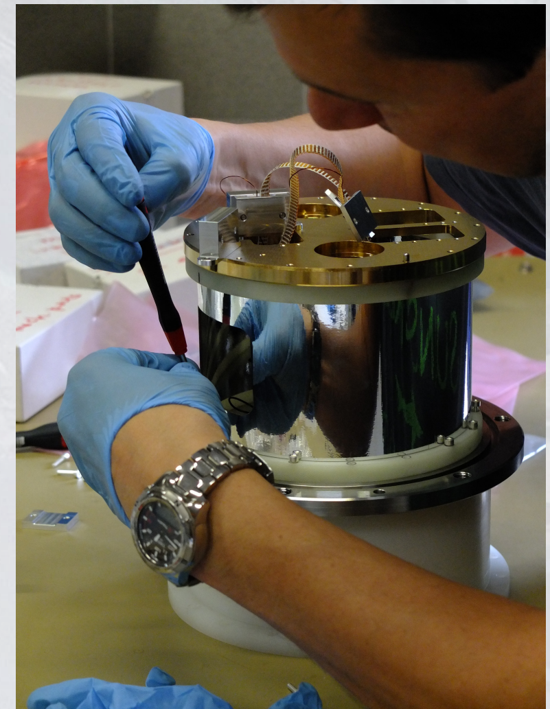
Integration of the Band 2+3 Cold Cartridge Assembly at IASF-Bologna
